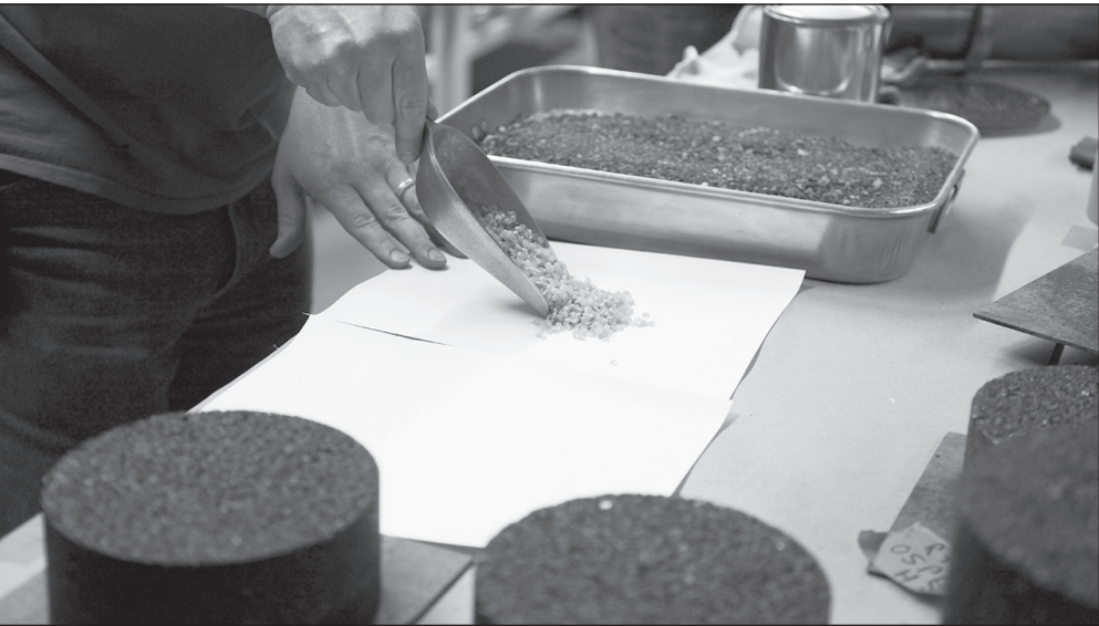
University of Missouri researchers are on the leading-edge of developing sustainable plastic waste road pavement mixtures. Lab staff in the Mizzou Asphalt Pavement and Innovation Lab, or MAPIL, show the plastic waste particles that are being added to the pavement mixture. The lab is located inside the MU College of Engineering. Contributed photo.
